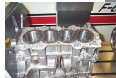
Honda block with AEBST sleeves installed on Rottler F65.
