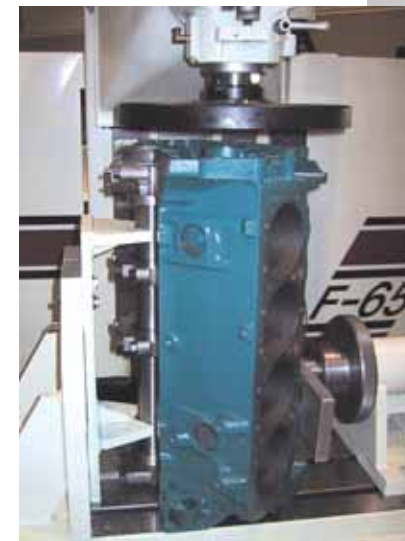
Honda block with AEBST sleeves installed on Rottler F65.
