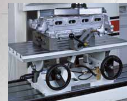
Rottler's patented 2 axis leveling table and universal quick clamping system for surfacing/ milling heads, blocks and manifolds with CBN and PCD tooling.
