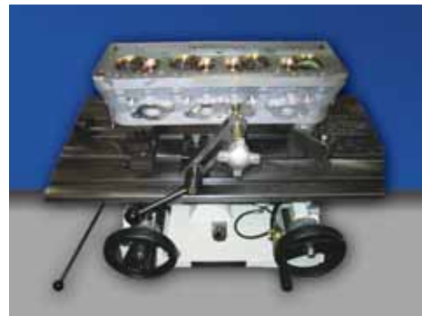
Dual axis leveling table for any style cylinder head or small inline blocks.
