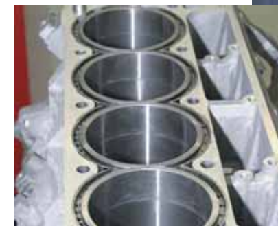
GM LS1 block with Darton MID sleeves installed on Rottler F65.
