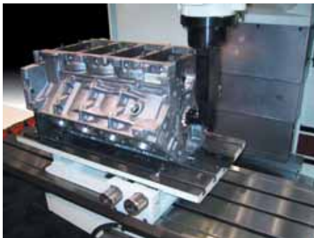
Pivot table for fast alignment when line boring, cam boring, stroker clearancing and machining for 4 bolt caps.
