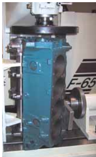
Pivot table for fast alignment when line boring, cam boring, stroker clearancing and machining for 4 bolt caps.
