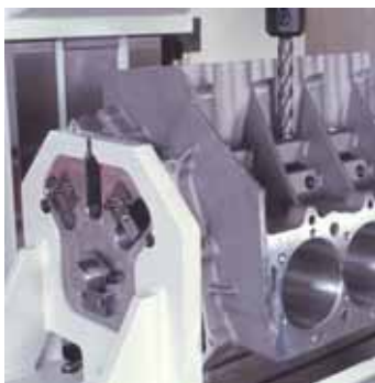
Precision fixture for blueprinting blocks, boring, decking, lifter bores.
