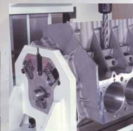
Lifter bore angles are accurately set with gage blocks in the Performance Fixture. Complete a lifter bushing job in less than one hour!
