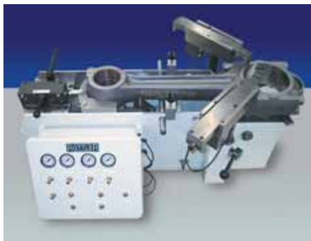
Connecting rod fixture for boring small and large ends of rods and controlling center to center distance.
