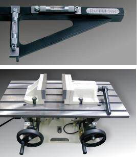
Two piece vice allows parts like exhaust manifold and main line bearing caps to be clamped, then leveled and
