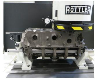
Extra clearance below and behind the fixture allow high deck height V-Blocks to be rolled to both banks for surfacing without removing the block from the machine.
