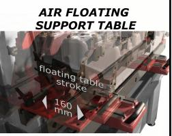
Cylinder heads up to 350 kgs can be moved back and forth without any effort and then locked by two powerful pneumatic jacks.
