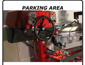
This extra length on the beam (optional) is available to ease the mounting and unmounting of large and heavy cylinder heads on the floating table.
