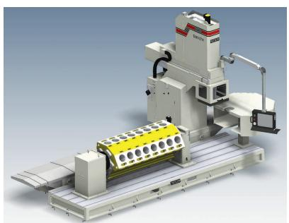
The size of the fixed worktable and traveling column design allows massive blocks/frames to be set up as well as multi work stations for set up of a variety of different parts or fixtures at one time. The extra long travel of the column allows a vertical lathe to be installed at one end of the machine so that large diameter parts such as wheel hubs and spindles can be turned increasing the versatility and redefining the phrase MULTI-PURPOSE.
