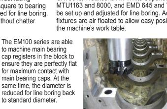
The EM100 series are able to machine main bearing cap registers in the block to
