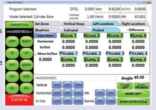
After centering is completed, touch –Auto Cycle – and the machine will automatically bore to the exact dimensions. These dimensions are saved under a block name for future use.
