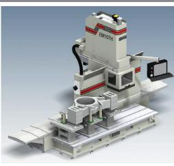
machine table and the machine table is likewise firmly anchored down onto the solid concrete floor. The workpiece is therefore stationary and the machine column moves left/right over the workpiece. This allows for very heavy and odd shaped fixtures and parts to be easily set up on the EM100 machines.
